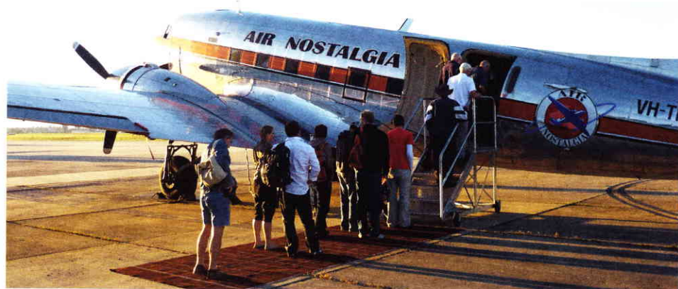
To date, the Flying Carpet boarding method has only been tested on passengers taking a pleasure flight on a vintage Douglas DC-3 Dakota. It appeared to work without any problems but this method can only really prove its worth if an airline/airport will trial it under today's commercial conditions. (Rob Wallace roundpeg@bigpond.com)
